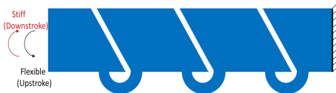
Figure 3. Conceptual Drawing of a 1 DOF Compliant Spine with 3 Compliant Joints
