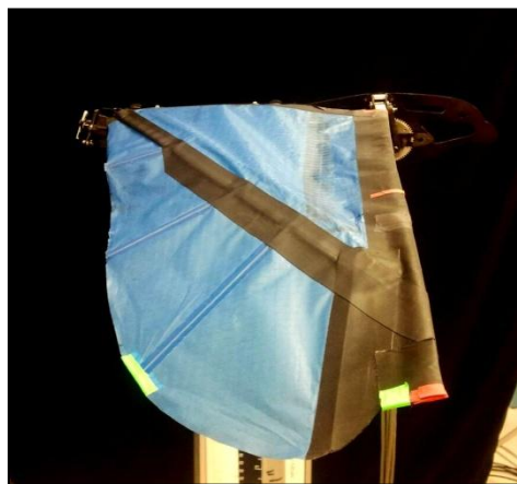
Figure 14. Marker Locations for Capturing Wing Twist Deflections
