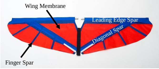
Figure 4: Top view of the research platform wings with its components labeled.
