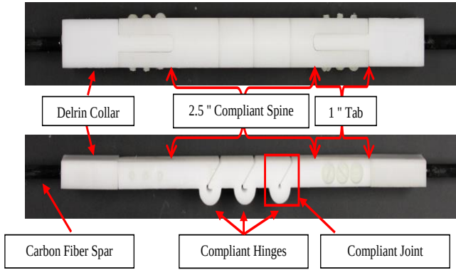
Figure 5. Compliant spine assembly components
