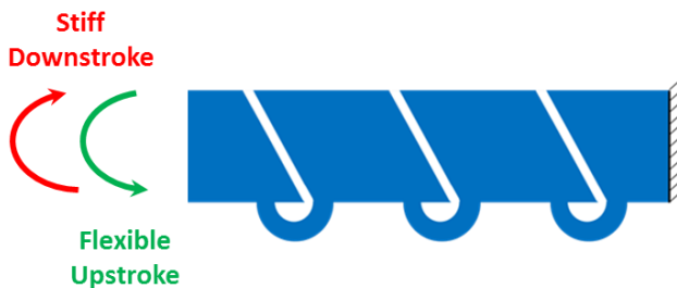
Figure 2. The desired stiffness of the compliant spine is nonlinear. It is stiff in the downstroke, similar to a rigid spar, and flexible in the upstroke, similar to a torsional spring.
